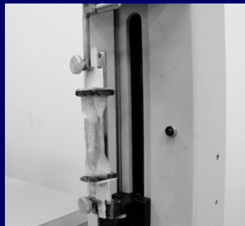
Uniaxial tensile test setup
