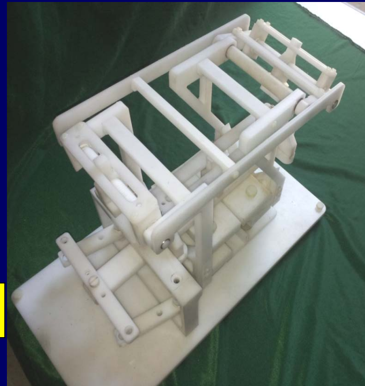
Fig.3 Virtual prototype of the surgical robot Fig.4 Physical prototype of the surgical robot
