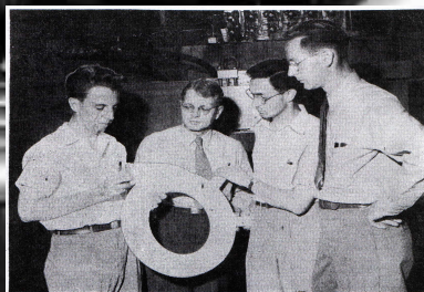
NEW ELECTRON BEAM DEVELOPED AT UI. A 22 million volt beam of electrons, which can smash into the atom in entirely new ways, has been produced from a betatron equipped with this new vacuum tube developed at the University of Illinois. In the projection is a "pedal" which deflects electrons from inside a tube and
