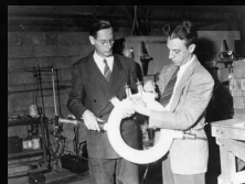
Kerst and Skaggs with the doughnut. Skaggs oints at the electron beam exit port. Med. Phys. 2, 1967 1975
