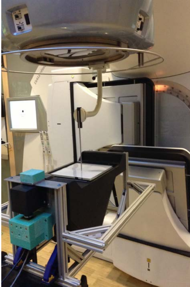
Suspended setup for gantry rotation measurements
